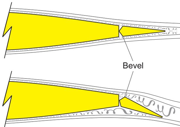
**Aileron example:** Due to the absence of smooth air flowing over the surfaces, small aileron deflections (stick movements) provide sluggish or erratic responses, especially at slower speeds. To begin achieving positive control, the pilot needs to apply larger inputs to deflect the surface up into the smoother air.
