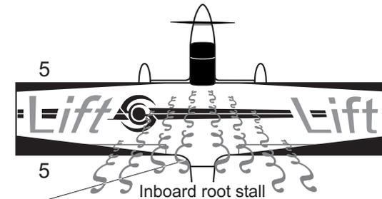
Stall: Airflow separates or no longer flows smoothly over the wing, resulting in loss of lift.
