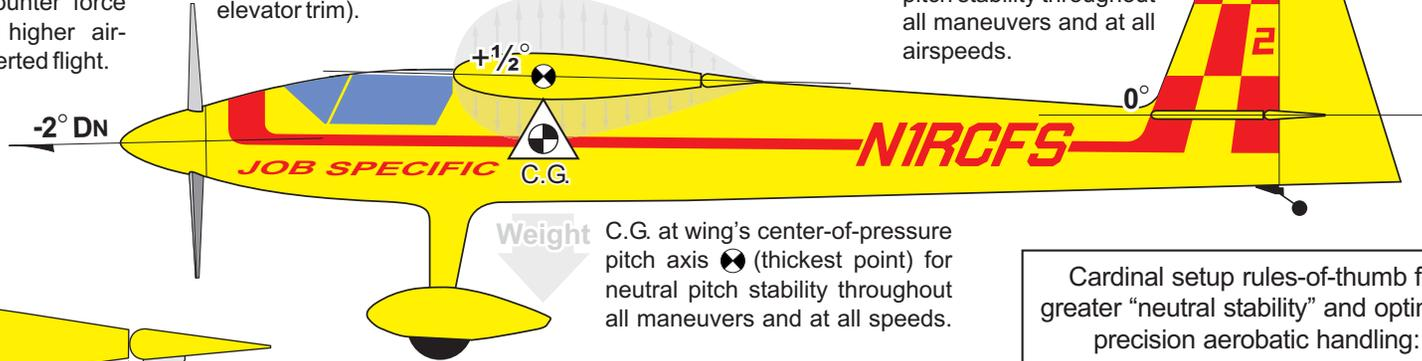
C.G. at wing's center-of-pressure pitch axis (thickest point) for neutral pitch stability throughout all maneuvers and at all speeds.
