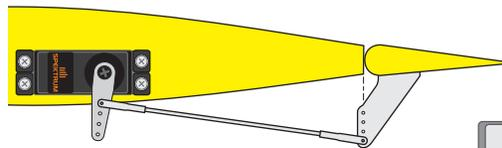
Pushrods connected to the holes closest to the servos and furthest out on the control horns to achieve maximum resolution (precision) and mechanical advantage (strength).
