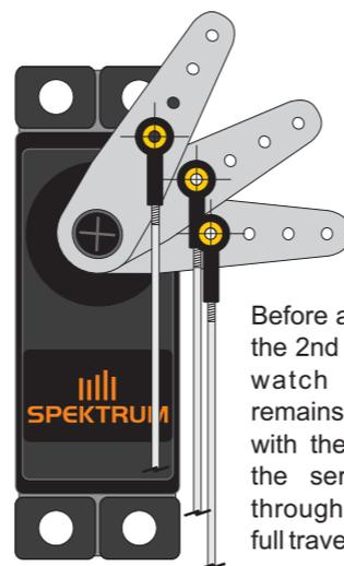
Before attaching the 2nd ball link, watch that it remains aligned with the hole in the servo arm throughout the full travel.
