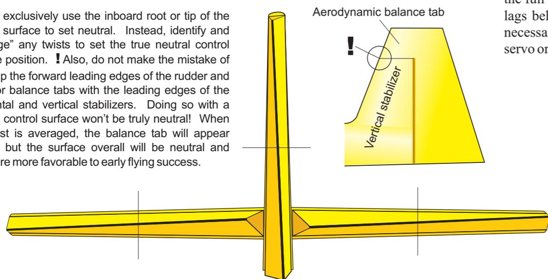
(Twisted elevator halves example) Despite one elevator looking like it is up, and the other down, they are actually both neutral when the twists are averaged.
