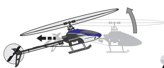
Elevator: Tilt Nose Up & Down
