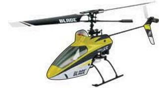
An entry level fixed pitch heli is inherently stable and returns to upright when the controls are neutralized. The more forgiving characteristics of fixed pitch helis translates to needing fewer aileron and elevator bump corrections to maintain a stationary hover.
