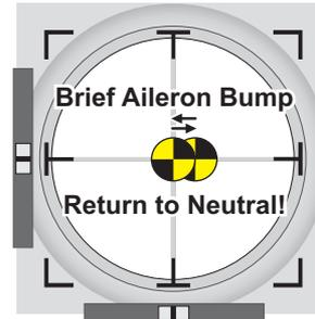
Small brief aileron & elevator bumps are the primary type of control input used to correct deviations during a stationary hover.
