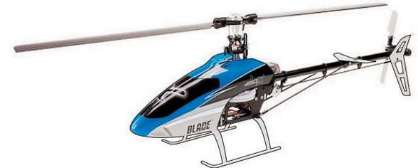
A collective pitch heli requires small brief aileron and elevator bumps during hover similar to those used to fly a fixed pitch heli, but because it’s less stable, constant corrections are required and there’s less margin for error if the right control stick is held in.
