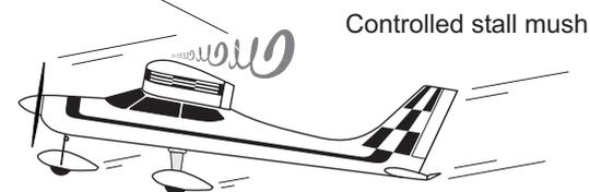
KPTR: The primary features of a good primary trainer are its flat-bottom airfoil, high wing placement and constant-chord.
