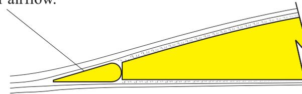
Notice: The airflow does not bump into the aileron's raised leading edge since the air is disturbed in that area.
