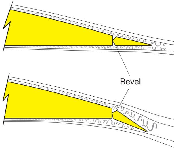
Note: The skin friction air disturbance and beveling increase the potential for control surface **flutter!**
