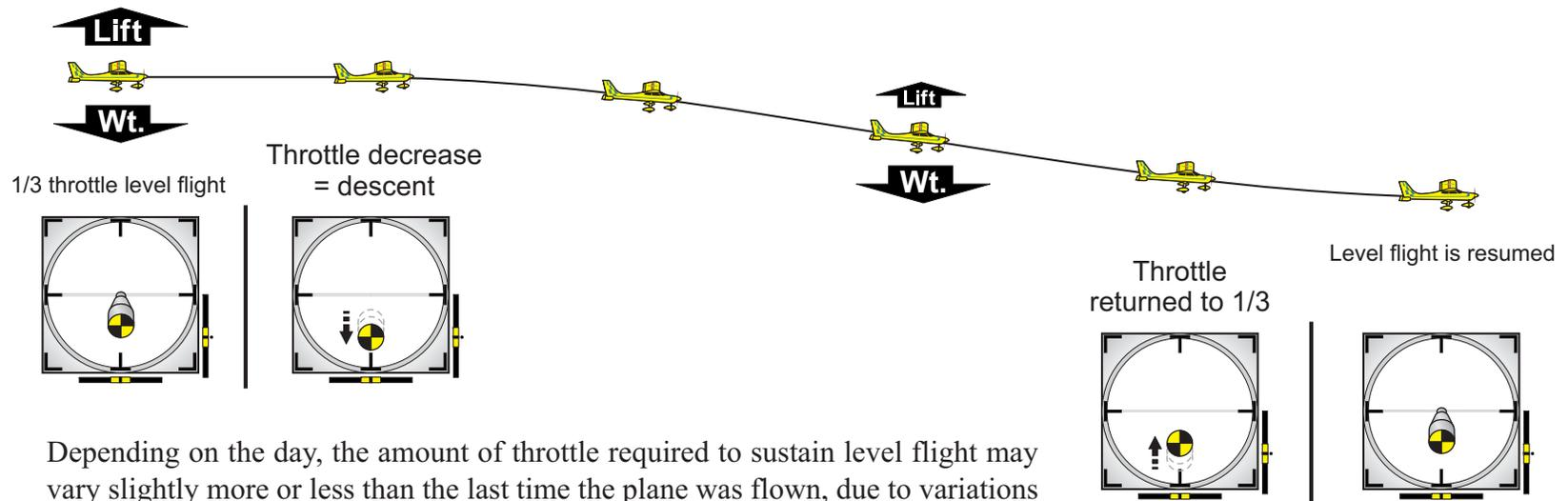
Depending on the day, the amount of throttle required to sustain level flight may vary slightly more or less than the last time the plane was flown, due to variations in temperature, humidity, etc.. In other words, each day the throttle should be close to 1/3, but not necessarily fixed right at.
