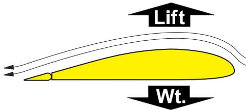
**When wing lift equals weight = level flight**
