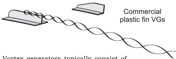
Vortex generators typically consist of small vanes or fins positioned near the wing leading edge that energize the boundary layer by creating vortices (tiny tornados) that pull fast-moving air down through the previously discussed stagnant or turbulent boundary layer near the surface. By energizing the airflow, VGs enable the wing to operate at higher angles-of-attack before stalling, provide gentler stall characteristics, and increase control and stability, especially at lower airspeeds.
