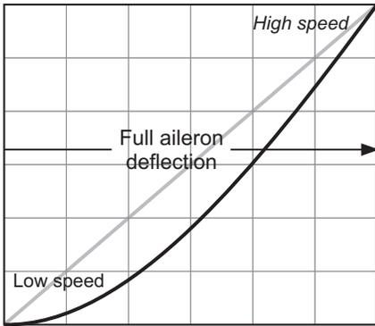
Traditional beveled surfaces produce an initial sluggish response and an irregular response rate that impairs a pilot's ability to predict how the plane will respond to commands, especially at lower airspeeds.
