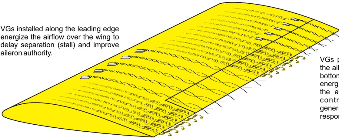
VGs positioned in front of the ailerons on the top and bottom of the wing re-energize the airflow over the ailerons to maximize control authority and generate a linear control response.
