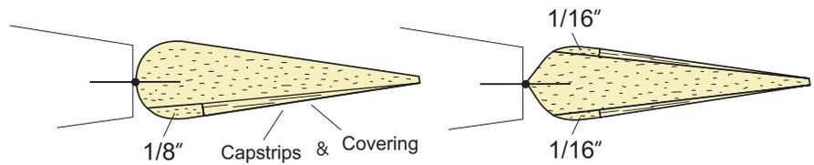
Rule-of-thumb: Raise the aileron, elevator, and rudder approx. 1/16" each side - 3/32" to 1/8" thicker overall.
