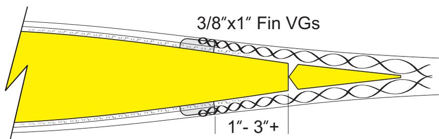
VGs installed along the leading edge energize the airflow over the wing to delay separation (stall) and improve aileron authority.
