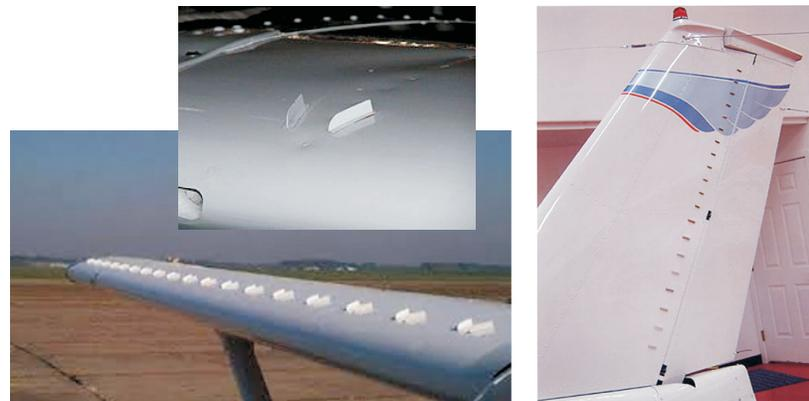
VGs positioned 1"-3" in front of the ailerons on the top and bottom of the wing re-energize the airflow over the ailerons to maximize control authority and generate a linear control response.
