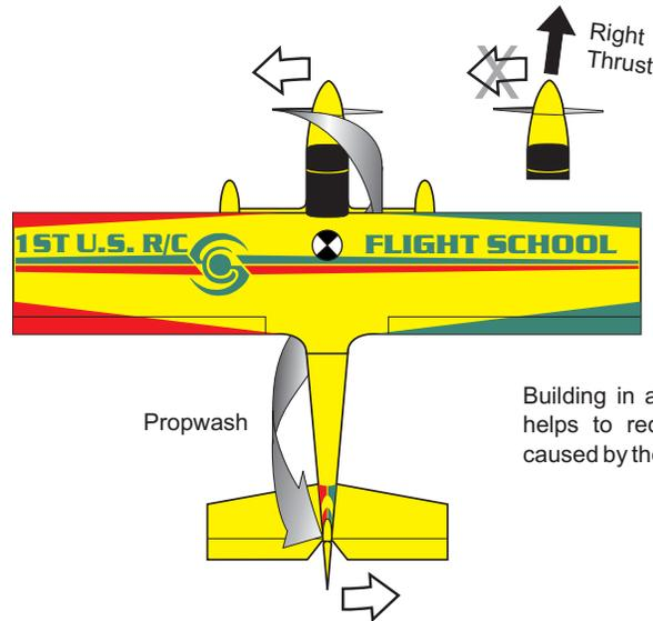
Building in a couple degrees of right thrust helps to reduce the left turning tendency caused by the propeller slipstream/propwash.
