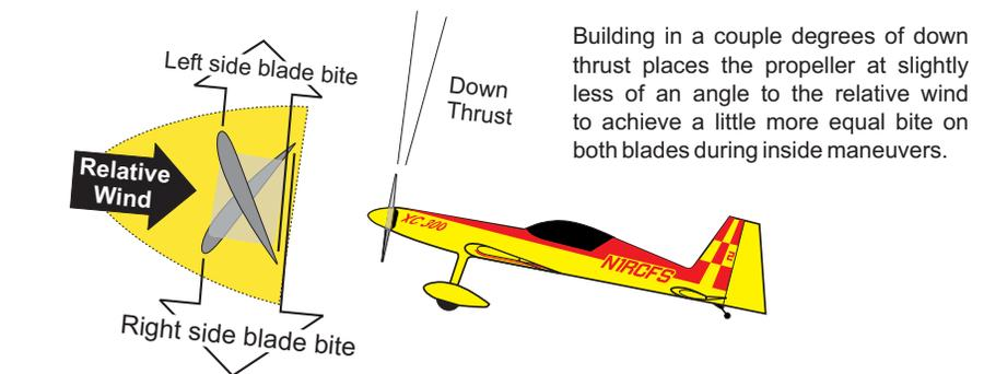
Building in a couple degrees of down thrust places the propeller at slightly less of an angle to the relative wind to achieve a little more equal bite on both blades during inside maneuvers.
