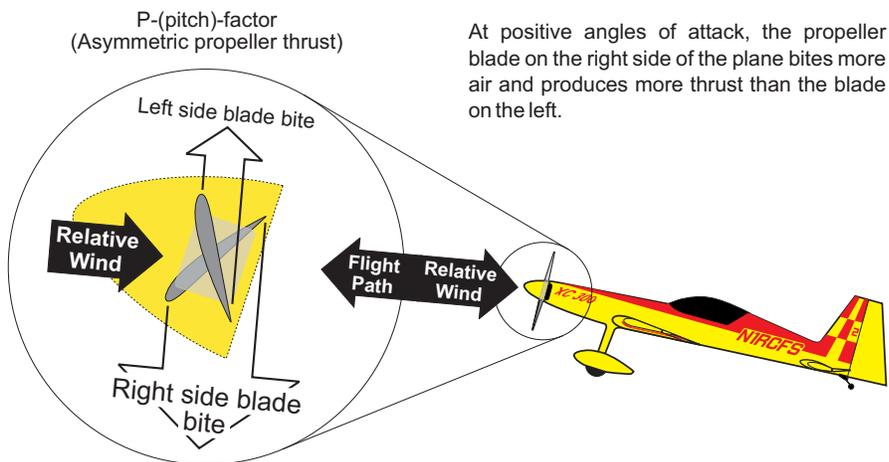
At positive angles of attack, the propeller blade on the right side of the plane bites more air and produces more thrust than the blade on the left.
