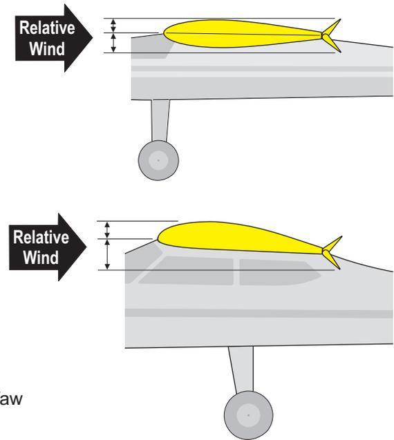
In flight, the down aileron presents a wider cross-section, thus increasing drag and causing adverse yaw, i.e., a yaw in the opposite direction that the ailerons are applied.
