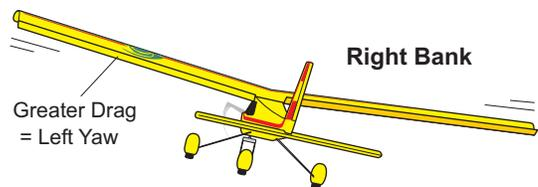
travel has little effect. To eliminate adverse yaw, rudder must be coordinated or mixed in the same direction with the aileron. As a rule, a symmetrical wing plane may require only a 3-5% rudder mix with the aileron to eliminate adverse yaw, whereas a flat
