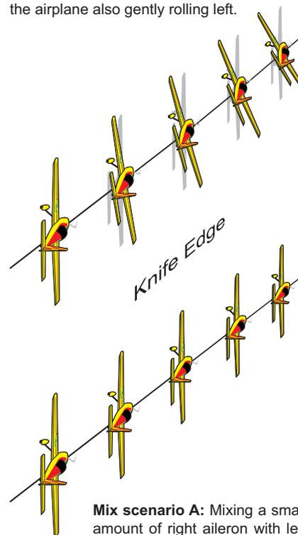
**Mix scenario A:** Mixing a small amount of right aileron with left rudder cancels the roll tendency during knife edge.
