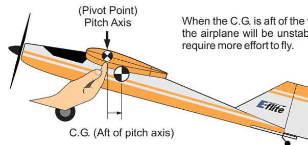
When the C.G. is aft of the wing's thickest point, the airplane will be unstable at all speeds and require more effort to fly.
