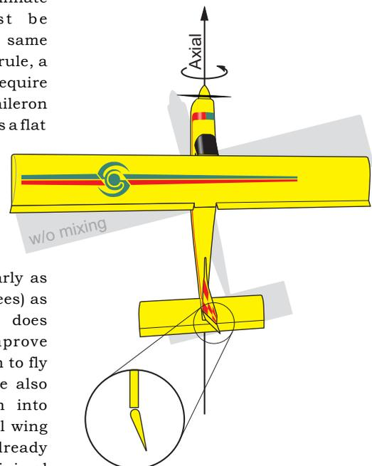
You must coordinate or mix rudder with the aileron in the same direction to eliminate adverse yaw when flying a flat bottom wing airplane.
