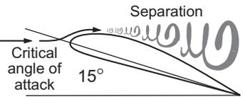
A stall or loss of lift occurs when the wing exceeds its critical angle of attack and the airflow becomes turbulent and separates from the wing.
