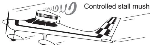
A constant chord wing inherently stalls at the root while the airflow continues to flow smoothly over the outboard portions of the wing. The resulting loss of lift at the root results in a controllable mush or sink while the tips continue to provide lift and aileron control during a stall.
