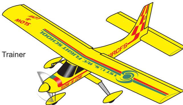
The primary features that make a good basic trainer are a thick flat-bottom airfoil, high wing placement and constant-chord.
